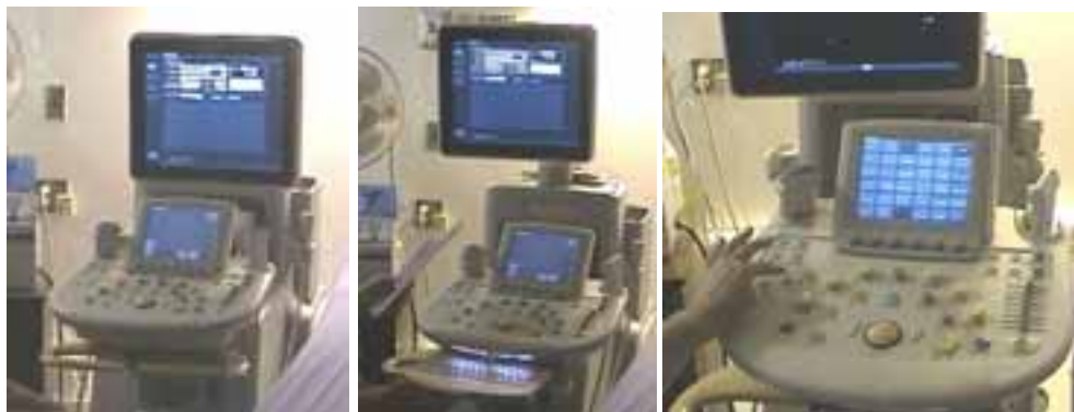
Figure 2, 3 and 4: These figures show some of the features on the newer ultrasound machine in Markdale (i.e. the adjustability, keyboard design, panel and touch screen layout).
