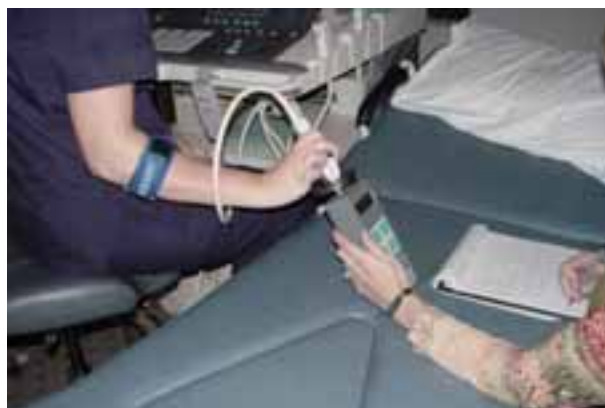
Figure 17: This figure shows the technique we used to measure/estimate the amount of force applied by the sonographer.
